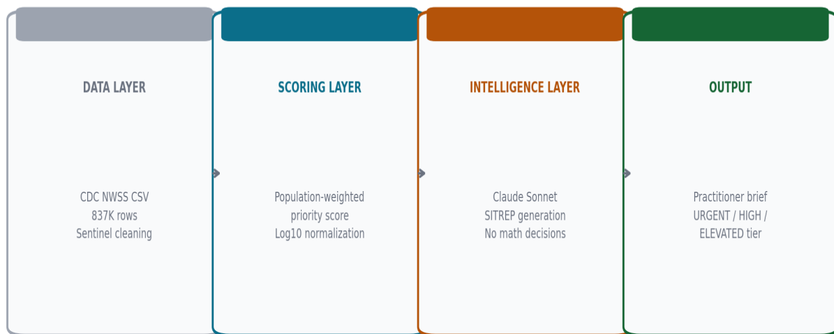
Figure 3 — BioSignal system architecture. Each layer has a distinct, non-overlapping role.
